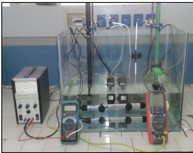
Fig. 2 Photo of the Installed ICCP System.
